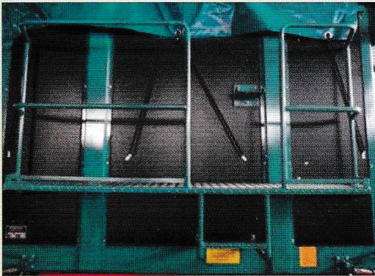
service platform on the front wall
